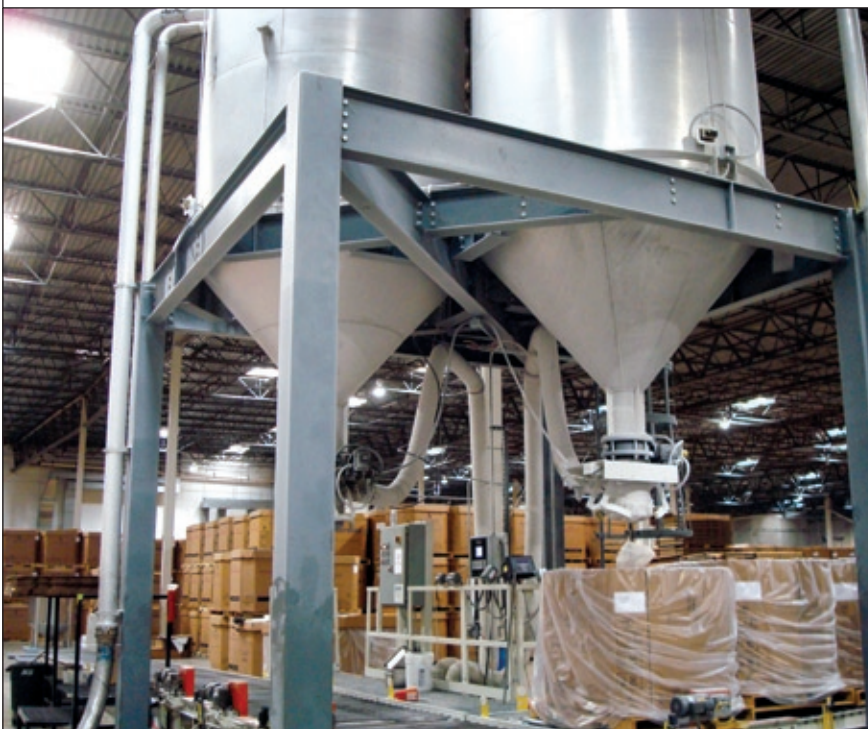
Next to a rail siding at the A&R Logistics facility, paired silos vacuum-suck plastic pellets from a rail car into boxes for packaging.
