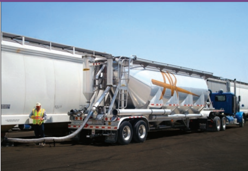
Pneumatic suction enables A&R Logistics to remove between 800 and 1,200 pounds of plastic pellets per minute from rail cars.
